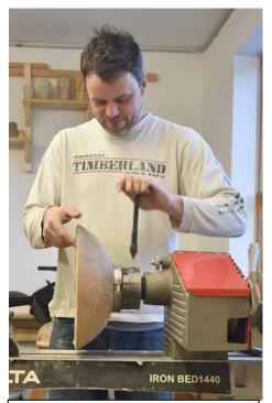
Nick feels the best way to deal with turning errors is to avoid them. He started with proper mounting on the lathe.
