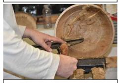
The tool is rotated to maintain the same cutting angle throughout the cut.
