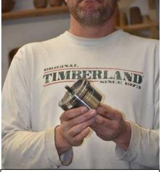
The "screw chuck" is held in a 4-jaw chuck. The work piece is screwed down to make contact with the jaws.
