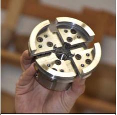
4-jaw chucks can have flat jaws or, like this one, dovetail-jaws. The bowl tenon should be cut to match the type of jaw.
