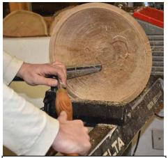
Making the interior cuts: The tool rest is close to the surface and below center enough so the tool is at center when presented to the wood. The tool bevel should ride on the wood and the cutting point back from the point slightly.
