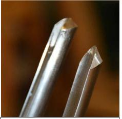
The bowl gouge on the left has a deeper flute than the spindle gouge on the right. Its cutting angle can be from 35 degrees to 75 degrees, depending on the wood you will use it on.
