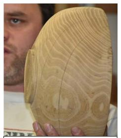
The tenon should be less deep than the chuck jaws. The bowl bottom at this stage should present a flat to the top of the chuck jaws.
