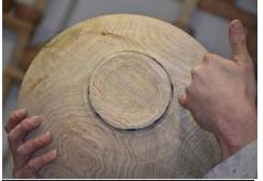
By cutting the tenon to fit the jaws, both inside and top, you get maximum bearing surface, and maximum grip. This resists having the workpiece pull away under heavy cutting.
