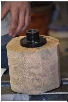
Faceplates are very safe. Nick uses decking screws, not drywall screws, as drywall screws can be brittle.
