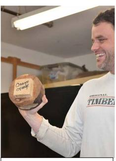
Another method, one which uses more of the "good" wood, is to glue a square of waste hardwood to the base of the workpiece. Sized properly, it is gripped by the jaws of the chuck. You could also screw a faceplate into it.
