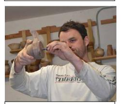
The "screw chuck" is another method of mounting to the lathe.
